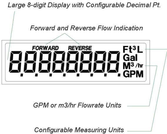
The following diagram shows the default display configuration for residential, commercial and industrial meters.
